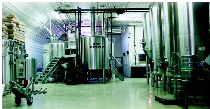
Huge stainless steel tanks and scientific instrumentation control the brewing process from raw ingredients to finished product.
